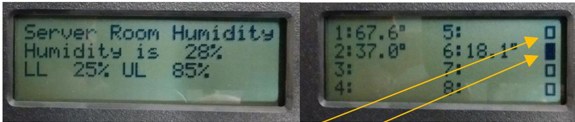
The dry contact inputs are on the right side of the display of the main screen. The open square means the input is **open**, a **closed** square is a closed input. Top square is Input #1, second is Input #2 etc. If the input is set to water sensor, the open square is no water detected, the closed square is a wet condition. The inputs are not displayed in the scroll through menu unless they are in alarm.
